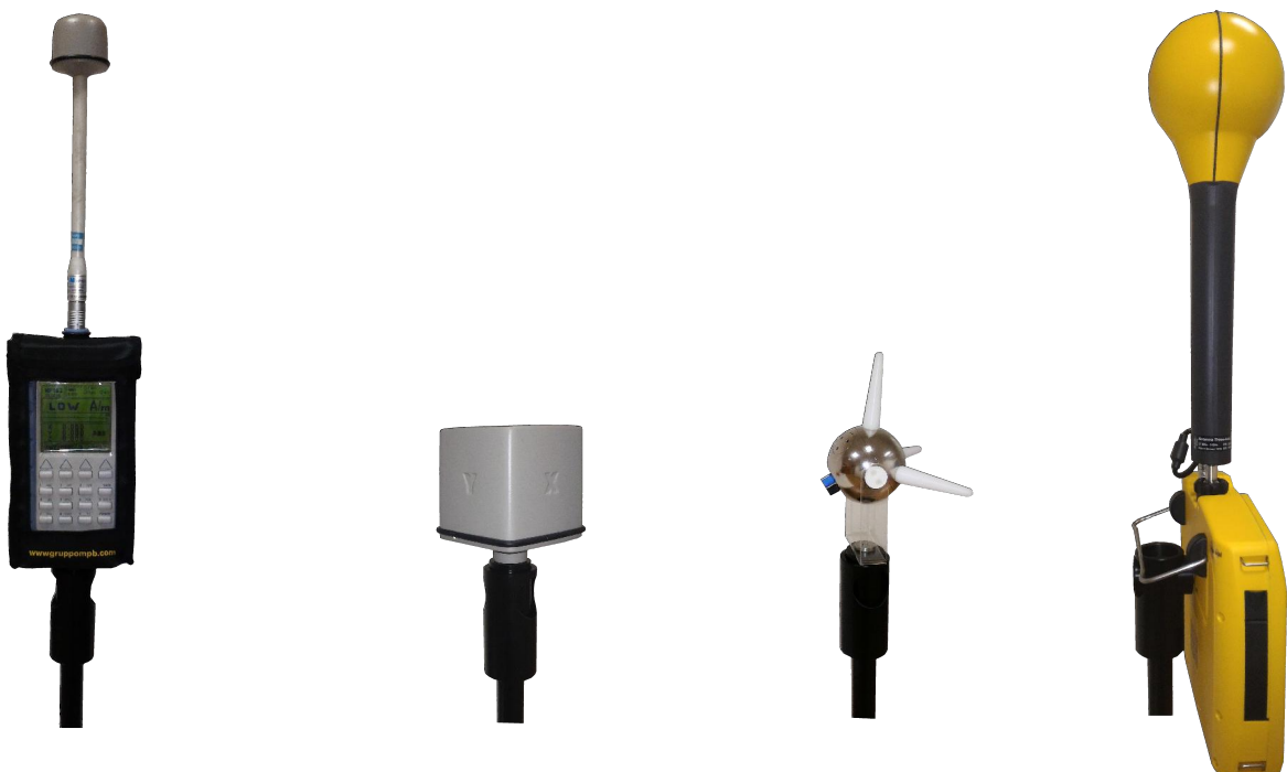
Vertical configurations for meters and antennas
